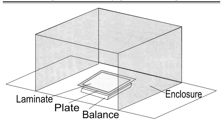
Figure 17.1. Typical Balance Enclosure
